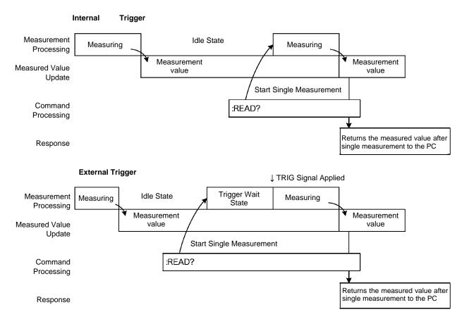
Use this method to measure (and export) synchronously with the controller (PC, PLC) or external trigger signal. Measurement time can be minimized.
