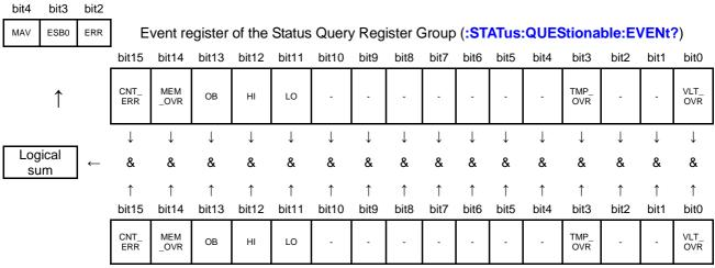
Enable register of the Status Query Register Group (:STATus:OPERation:ENABle)
