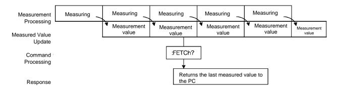
This is the simplest method for exporting measured values. It is ideal when measurement (tact) time is not limited, and when external synchronization is not needed. After connecting to the measurement target, wait for twice the measurement time before exporting the measured value.
