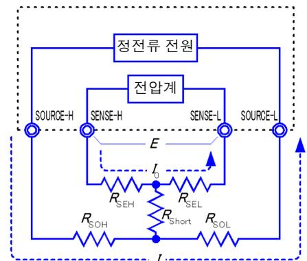
$$\begin{aligned} E &= (I_0 \times R_{SEL}) + (I_0 \times R_{SEH}) \\ &= (0 \times R_{SEL}) + (0 \times R_{SEH}) \\ &= 0 \text{ [V]} \end{aligned}$$
